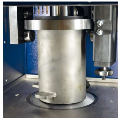
Compaction phase: simultaneous action of a static compression and of the shearing action
