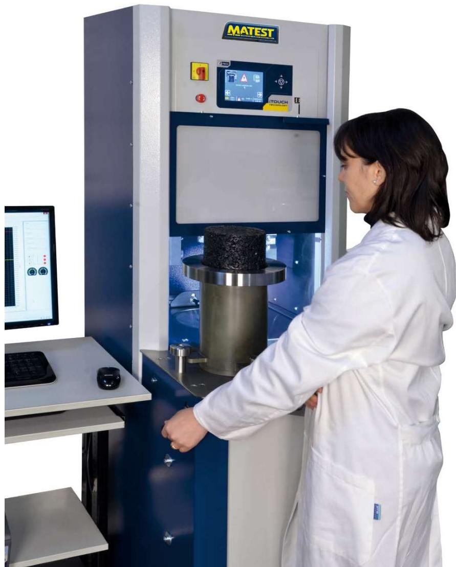
Test execution with shear stress measurement
